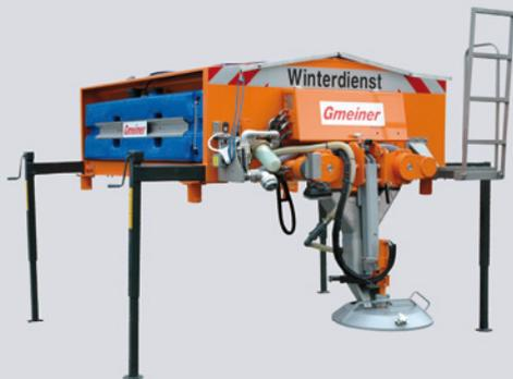
Supplied in container sizes 1.8 m<sup>3</sup> to 4.4 m<sup>3</sup> with and without wet salt equipment.
